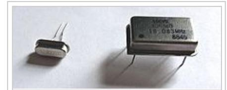
Quartz crystal resonator (left) and quartz crystal oscillator (right)
