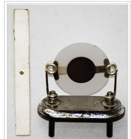
Flexural and thickness-shear crystals
