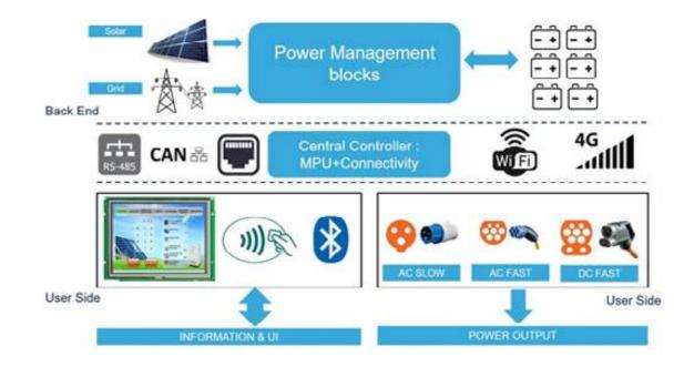
There is the user side, which basically depicts the functionalities visible to the end user. Information exchange and the user interaction is taken care of, here. It would typically consist of a TFT screen with touch sensing, <u>NFC</u> card readers for authentication or payments, and also a <u>Bluetooth</u> interface for more advanced features.
