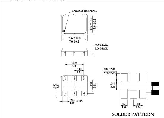
\*0.01µF external by-pass filter is recommended as shown on solder pattern.
