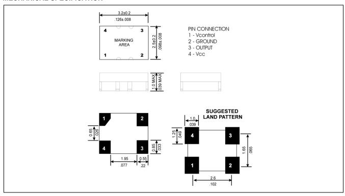
NOTE: Add a 1000 pF DC-cut capacitor to the output pad of the TCXO.
