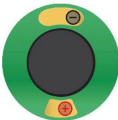
Electrical contacts of the MEMS speaker.
