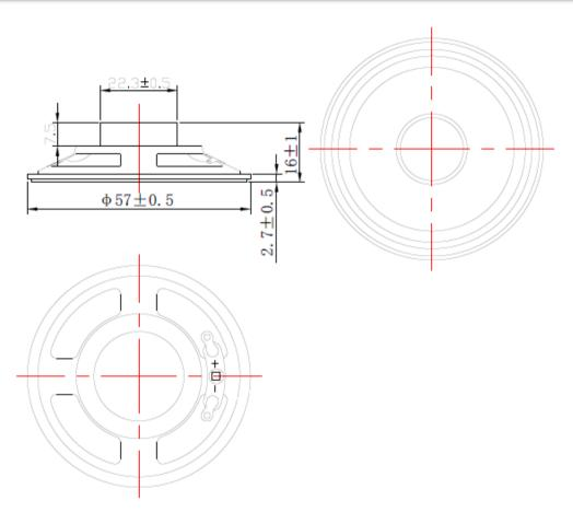
Unless otherwise specified,tolerance: ±0.5(unit:mm)
