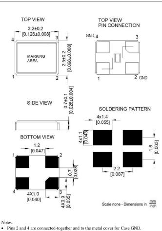
Pins 2 and 4 are connected-together and to the metal cover for Case GND.
