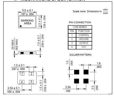
NOTE: A capacitor of 0.01  $\mu F$  between Vcc and Ground is recommended
