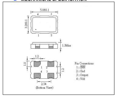
NOTE: A capacitor of 0.01 µF between Vcc and Ground is recommended
