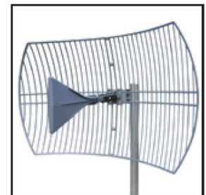
12) Completed Antenna NOTE: The antenna has a very narrow radiation beam. Antenna will only work within the narrow signal cone.
