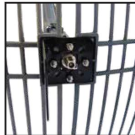
7) Secure the left & right bolts in place to hold bracket. Then proceed with remaining bolts for top & bottom of feedhorn.
