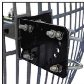
10) Once on mast, secure nuts on U-bolt. L-bracket allows for vertical alignment in combination with holes & the U-bolts.
