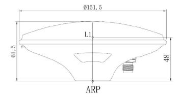
Mechanical Offsets Units in "mm"
