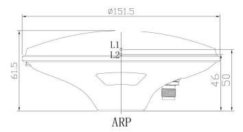
Mechanical Offsets Units in "mm"
