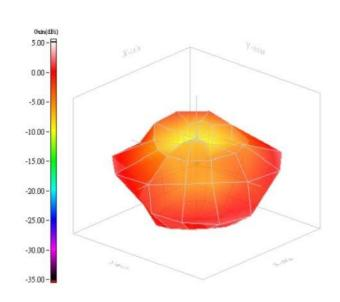
Max gain= 1.67dBi, at (90, 150) MEG (mean effective gain)= -2.69dBi Directivity(dB)= 3.87 Efficiency= -2.20dB, 60.30%
