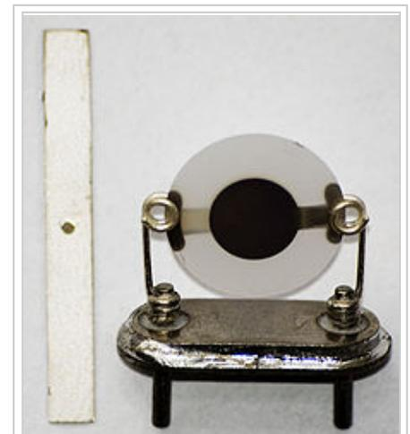
Flexural and thickness-shear crystals
