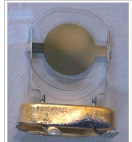
Inside construction of a modern high-performance HC-49 package quartz crystal
