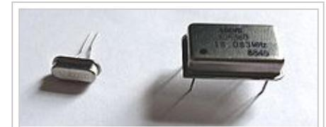
Quartz crystal resonator (left) and quartz crystal oscillator (right)
