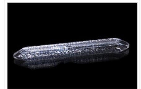
A synthetic quartz crystal grown by the hydrothermal synthesis, about 19 cm long and weighing about 127 g
