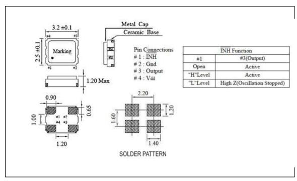
NOTE: A capacitor of 0.01  $\mu F$  between Vcc and Ground is recommended
